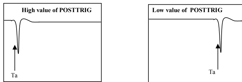
Fig 3a : centering of the Trigger in the acquisition window for two POSTTRIG cases.
